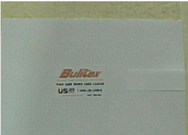
5. Heat iron to 430°, position over the repair area and apply pressure for 45 seconds.
