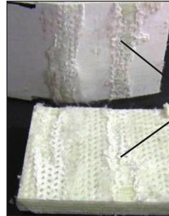
Failure mode at interface and scrim layer indicated that the 2-line Ultra-Sonic weld was very weak. Ultra-Sonic weld line acts as a crease which concentrates the forces and allows easy bending and pre-cracking, further weakening the assembly's integrity. In addition, the top connection between wall and scuff is "NOT" welded leaving areas for material and moisture build-up.
