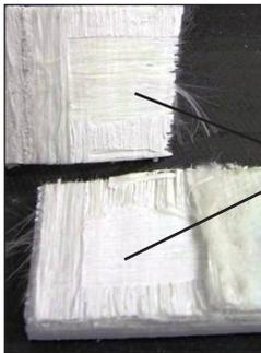
The cohesive failure of substrate indicated that the bond is stronger than the substrates themselves.
